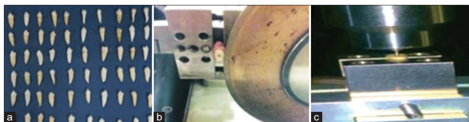
Figure 1: (a) Mandibular premolars selected for the study. (b) Specimens sectioned using an Isomet device (c) Push out bond strength tested on a universal testing machine
