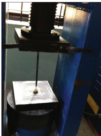
Figure 1: Fracture resistance test of specimens using universal testing machine
