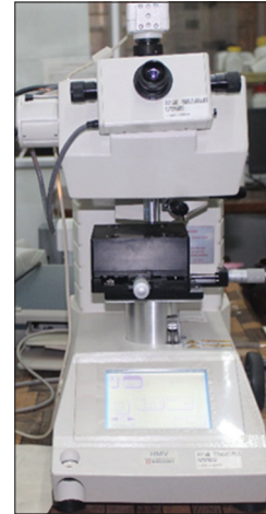
Figure 8: Micro Vickers hardness tester (HMV SCHIMADZO, model-HMV 2T ADW)
