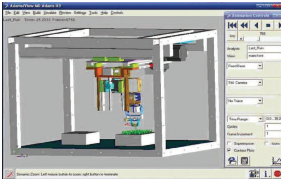
Figure 4: Virtual prototype for tooth-arrangement robot of Cartesian type
