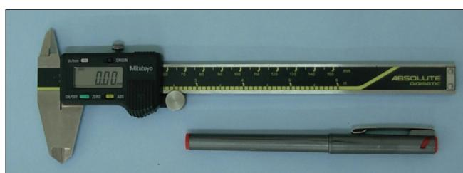
Figure 1: Digital vernier caliper used in the study
